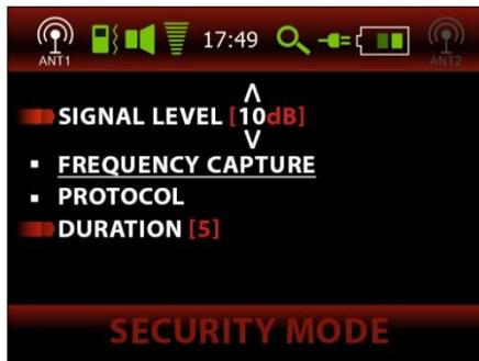
Fig.19 – Relative threshold signal level change for alarm engagement
