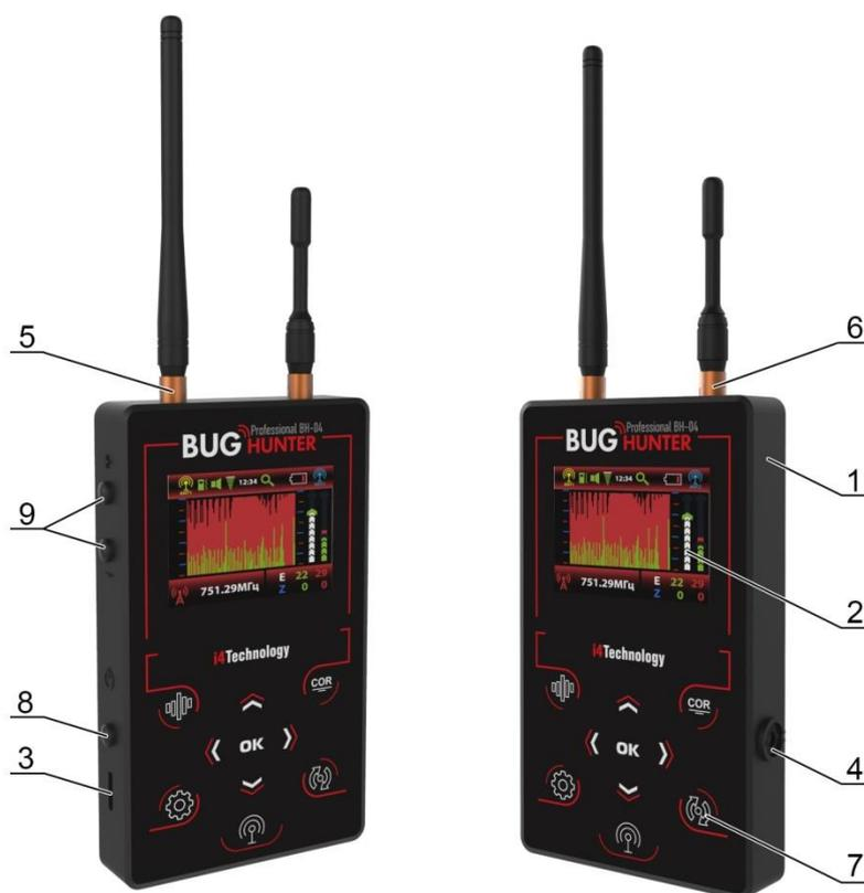
Fig.2 – Scheme of the main components
